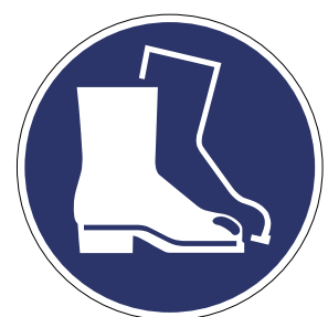
Use foot protection (ASR A1.3)
