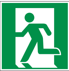
Escape route left (ASR A1.3)
