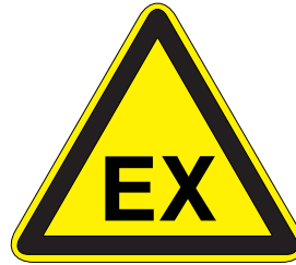
Warning of explosive atmosphere (ASR A1.3)
