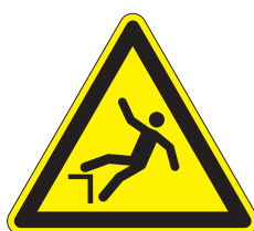
Risk of falling warning (ASR A1.3)
