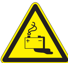
Warning about danger through charging batteries (ASR A1.3)
