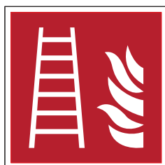
Fire escape F003
