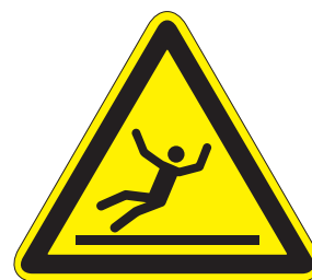
Risk of slipping warning (ASR A1.3)
