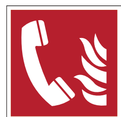
Fire alarm telephone F006
