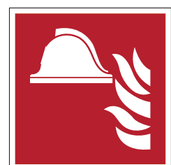
Means and equipment for firefighting F004
