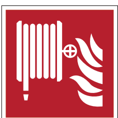
Wall hydrant F002
