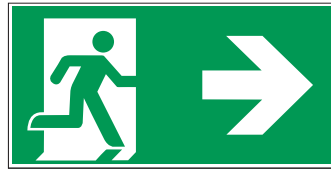
Emergency exit right (ASR A1.3)
