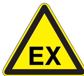
Warning of explosive atmosphere (ASR A1.3)
