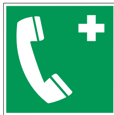
Emergency telephone E004
